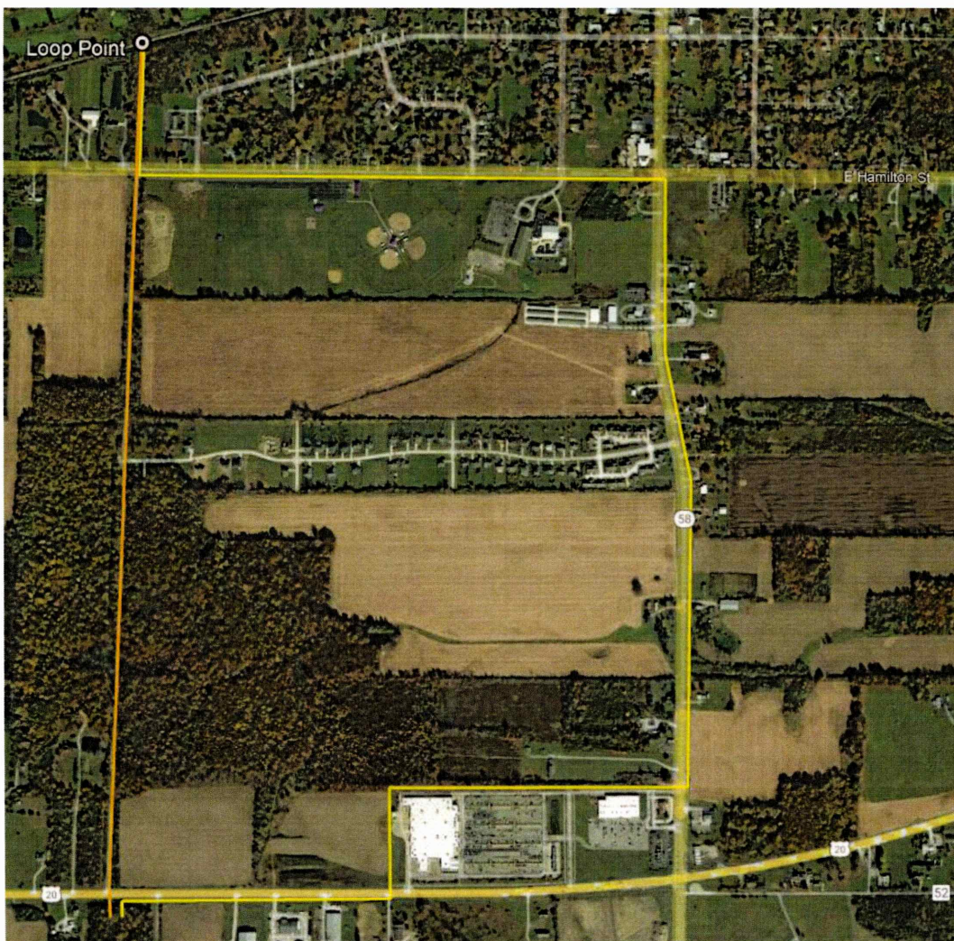
Figure 1. Transmission pole-line route options to create loop to new sub between the Power Plant and Switching substations.
