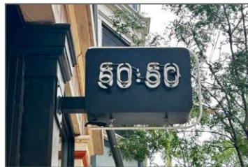
Figure 26: Graphic showing business sign using channel letters illumination. In this case, the channel letters are produced by neon tubes, but this is not always the case.
