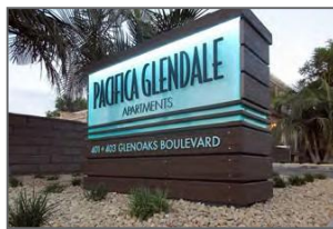
Figure 28: Graphic showing business sign using halo-letters illumination.
