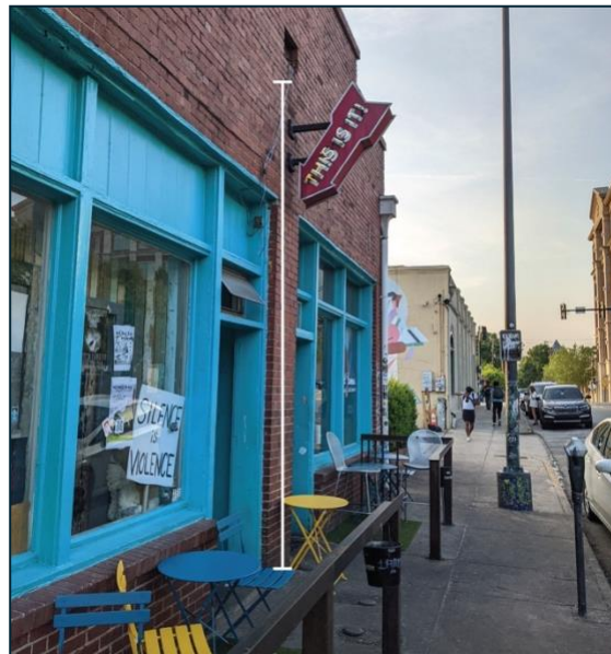
Figure 25: Graphic showing sign height reaching from average grade of the ground up to the top of the decorative part of the sign (white line). In this image, the sign is a type of Projecting Sign.
