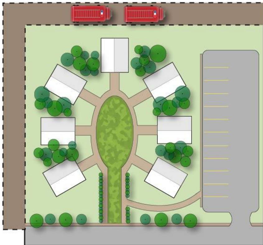
Figure 19: Graphic showing fire access via a fire lane (an option but not required) for a cottage court
