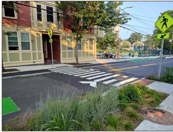
Figure 9: Graphic showing raised pedestrian walkway crossing vehicular right-of-way
