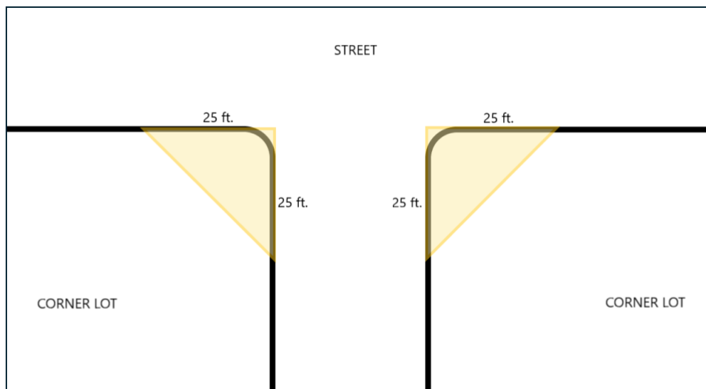
Figure 22: Diagram showing the Vision Clearance Triangle for corner lots.
